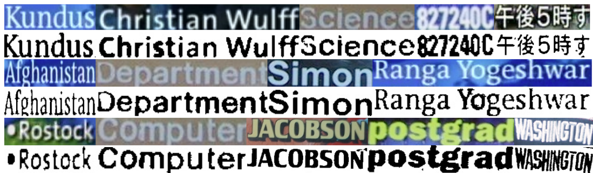
Fig. 4. Some example binarization results of our method from German TV news test set and ICDAR 2003
