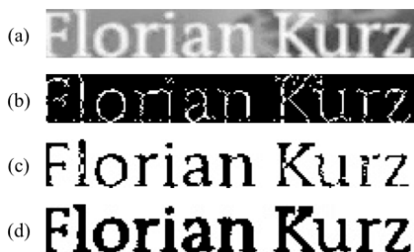
Fig. 3. Seed selection and region growing results: (a) grayscale image, (b) skeleton image, (c) seed image, (d) region growing result.
